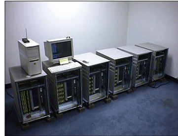
DES Keysearch Machine, 1998 (Cryptography Research, AWT, EFF) Tests 90+ billion keys per second, exhaustively searches 56-bit DES keyspace in 9 days.
