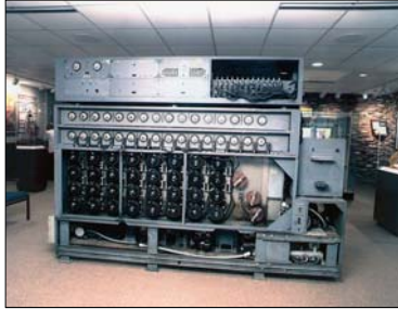
US Navy Bombe, 1943 Contains 16 four-rotor Enigma equivalents to perform exhaustive key search.
