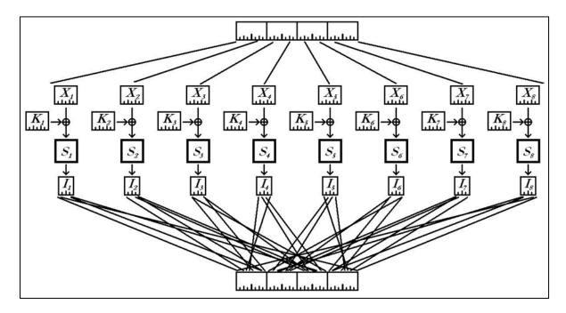
The 32 bits are expanded to 48 bits, and grouped into eight 6-bit blocks. As with AES, each block  $X_j$  is XORed with a block of key  $K_j$ . The results of the XORs are then transformed by  $6\rightarrow 4$  bit lookup tables  $S_j$ . The bits of the resulting intermediates  $I_j$  are then permuted, and the permuted bits are then XORed with the other 32 bits of the data (not shown), to complete the round.
