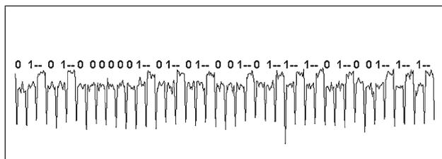
**Fig. 11** SPA leaks from an RSA implementation
