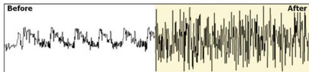
**Fig. 21** Example of adding amplitude noise to obscure and reduce signal (simulated data)
