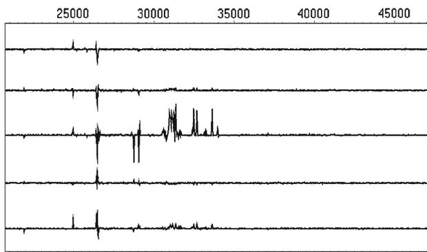
**Fig. 8** Five differential traces for the DPA test predicting the LSB of  $I_{i,0}$  for guesses  $K_0 = 101, \dots, 105$  from top to bottom, with the correct key  $K_0 = 103$ , corresponding to the third trace
