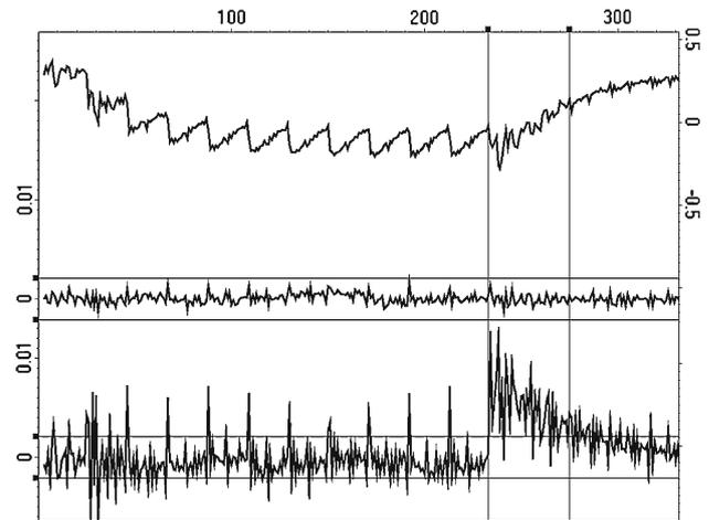
**Fig. 9** DPA results showing the average trace for an AES-128 operation running on an FPGA (top), the differential trace for an incorrect guess of a byte of the last round key (middle) and the differential trace for the correct key byte (bottom)
