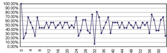
**Fig. 17** Biases observed for incorrect key guesses of DES S-box 2, output bit 2. The X axis shows the XOR difference between the tested 6 key bits and the correct key bits. The Y axis shows the likelihood the incorrect key will correctly predict the output bit
