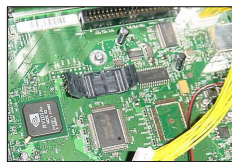
BIOS socket (X-Box) Bunnie Huang, xenatera.com
