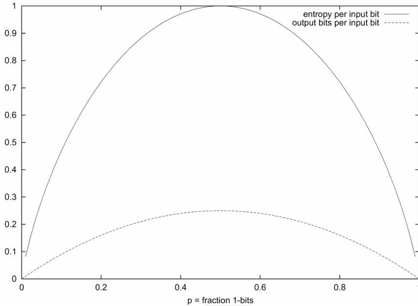
**Figure 10: von Neumann correction of biased, independent bits**
