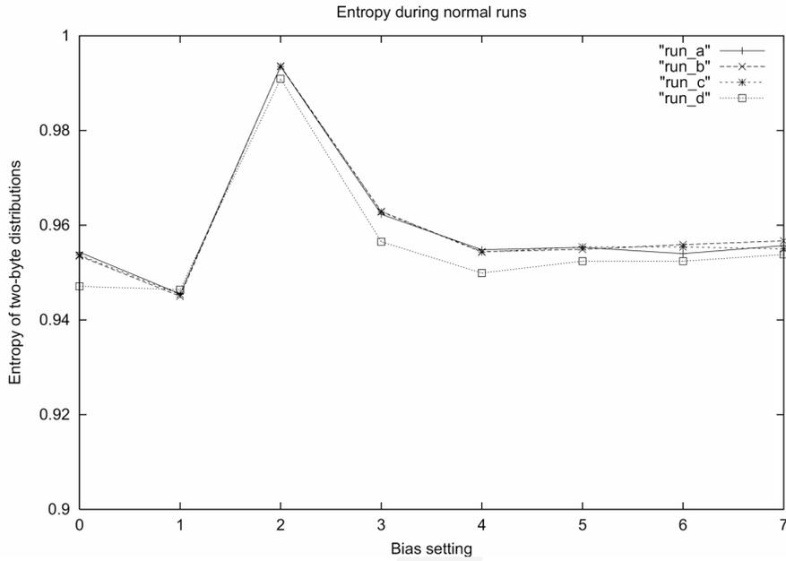
Figure 3: Entropy during continuous RNG operation (raw output)
