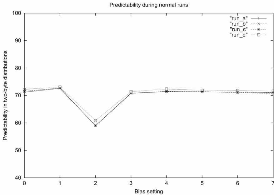
Figure 4: Predictability during continuous RNG operation (raw output)
