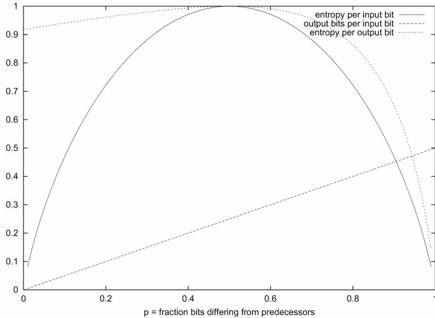
**Figure 11: von Neumann correction of serially correlated bits**
