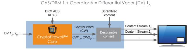
Single CryptoFirewall core simultaneously supports multiple CAS/DRM and operator combinations
