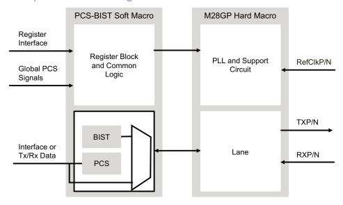
We offer complete PHY solutions – our SerDes PHY includes a Physical Media Attachment (PMA) hard macro and Physical Coding Sub-layer with Built-in Self-Test (PCS-BIST) soft macro. The PHYs can also be configured to multiple channel widths and packaging options, which simplifies integration and maximizes design flexibility.
