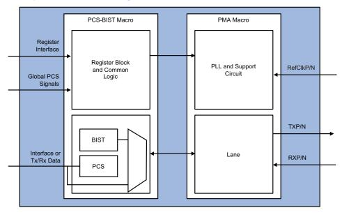
We offer complete PHY solutions – our SerDes PHY includes a Physical Media Attachment (PMA) macro and Physical Coding Sub-layer with Built-in Self-Test (PCS-BIST) macro. The PHYs can also be configured to multiple channel widths and packaging options, which simplifies integration and maximizes design flexibility.
