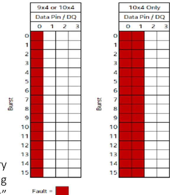
Figure 2: Fault boundary for DDR5-BF x4 devices. In all 9x4 devices major sub-CL faults will impact data on one DQ. Major sub-CL faults in 10x4 devices can impact data on either one or two DQs.
